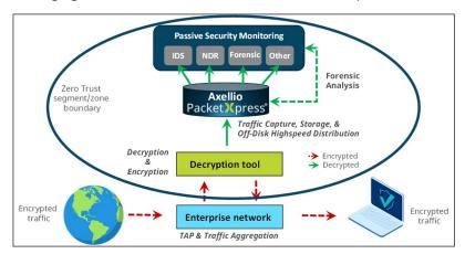
The Axellio solution handles data processing, data buffering, data storage, and data transmission to the security tool functions. This creates a simple, cost-effective, and completely secure threat detection and analysis solution for enterprise networks.
